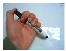
*Correct Method: Use index finger and thumb to control dispensing plunger.*
